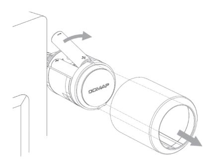
! Change the batteries while observing the polarity engraved on the plastic housing.
